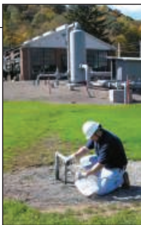
FIGURE 2. (above) In field-sampling, some parameters must be analyzed onsite because of their time-dependency
