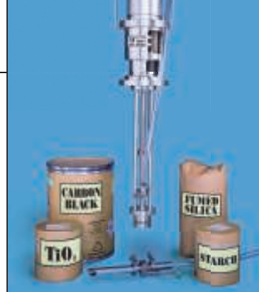
FIGURE 7. This batch-configured high shear mixer is equipped with a wand and feed tube that terminates beneath the surface of the batch. Powders are sucked through the tube and injected directly into the high shear zone, where they are dispersed instantly
