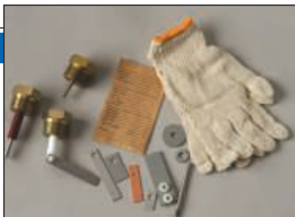
FIGURE 4. Metal coupons of known weights can be installed into the pipeline to determine weight loss by corrosion over time
