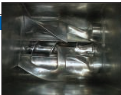
FIGURES 3 and 4. Sigma blade mixers (above) apply great power to mix materials at extremely high levels of viscosity. Recently, however, innovative helical blades (right) have extended the working viscosity of double planetary mixers significantly. This has made many high-viscosity applications appropriate for either a sigma blade mixer or a planetary mixer
