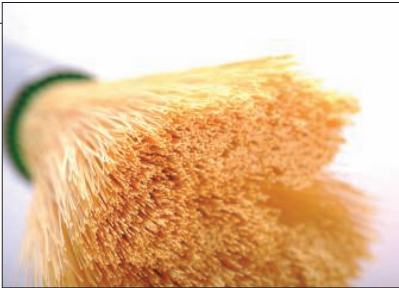
FIGURE 3. Modules of these spaghetti-like hollow-fiber membranes can upgrade biogas to a CH 4 purity of 99%
