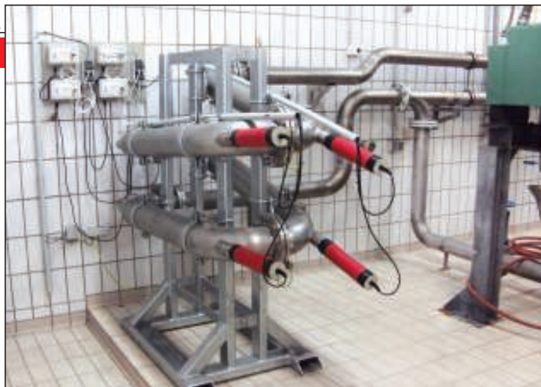
FIGURE 2. Biogas yields can be increased by up to 15% by adding BioCrack electrokinetic disintegration modules
