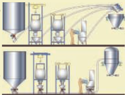
FIGURE 1. Mechanical (above) and pneumatic (below) gain-in-weight batching systems can transport material from silos, manual dumping stations, process equipment, bulk bags or any other source to a hopper, a blender, or other downstream equipment mounted on load cells
